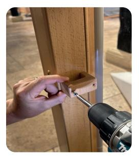
2. Screw the hand control hook in place using the enclosed screws.
